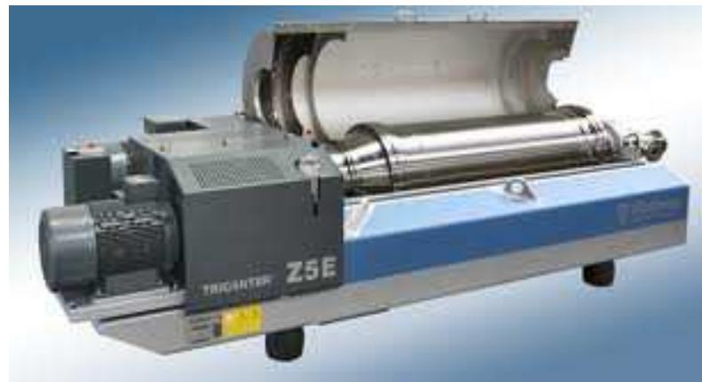
Olive oil extraction by Decanter centrifugation
