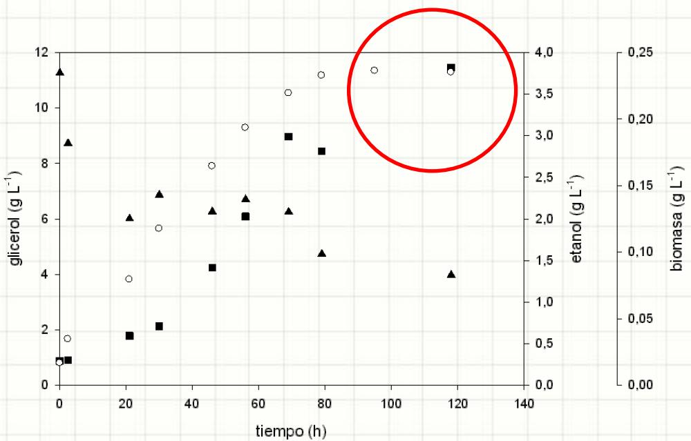
Profiles of fermentation obtained for R5BGFGAr (initial concentration of glycerol 10 g L<sup>-1</sup>, 37°C, 150 rpm, pH=6,3). (■) ethanol, (▲) glycerol, (○) biomass.
