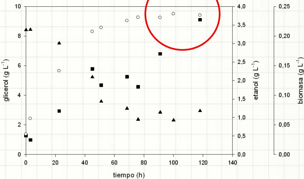
Profiles of fermentation obtained for R5BGCAr (initial concentration of glycerol 10 g L<sup>-1</sup>, 37°C, 150 rpm, pH=6,3). (■) ethanol, (▲) glycerol, (○) biomass.
